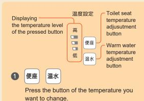
2 Press the button selected in step 1 repeatedly until a desired temperature level lights up.
