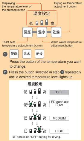
If the button is not pressed for about 10 seconds, the temperature adjustment LED will go off, but the setting will be retained.
